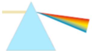
Fig. 5b. Light disperses as it passes through a prism made of fluorite. Notice that, compared to light passing through a glass prism, light of different colors is much less spread out.
