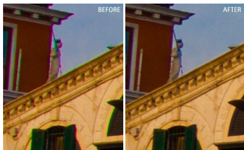
Fig. 6a. Different colors of light bend at different angles when they pass through a glass lens, resulting in chromatic aberration.
